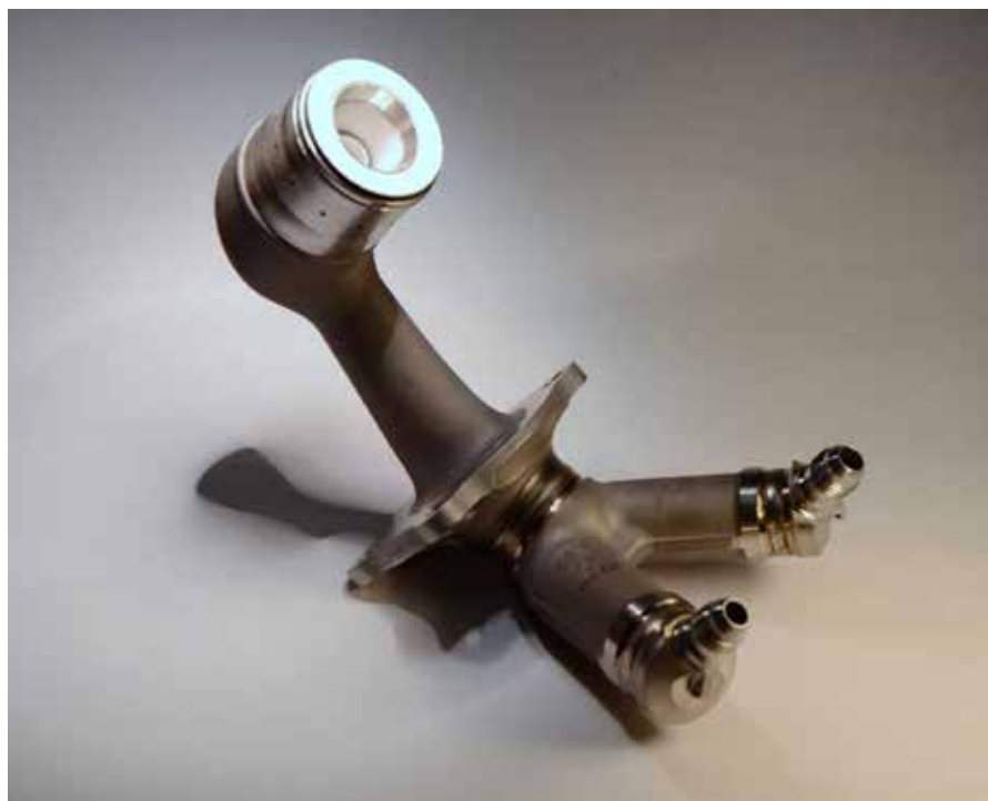
Fuel injector for the GE LEAP engine, produced as a single piece using AM, which traditionally consisted of 20 parts (Source: General Electric)
