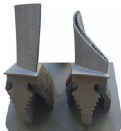
Cross-section of a turbine blade produced by AM using Laser Powder Bed Fusion (LPBF), showing internal cooling channels. (Source: https://doi.org/10.1007/s12541-024-01177-3 )
