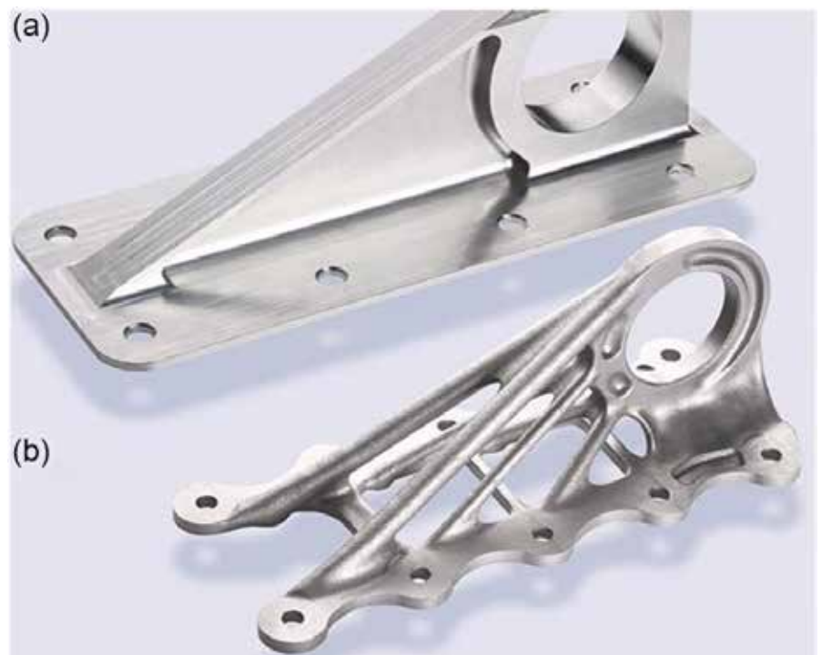
Titanium cabin bracket produced by a) Traditional and b) Additive Manufacturing methods (Airbus A350 XWB. Copyright 2023, Elsevier.)
